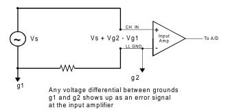
Single-ended input with Common Mode Voltage
